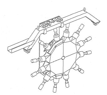
Figure 1. Perspective view of the new 6-inch thick scintillation detector being constructed at IUCF showing all four quadrants and part of the mechanical support structure.
