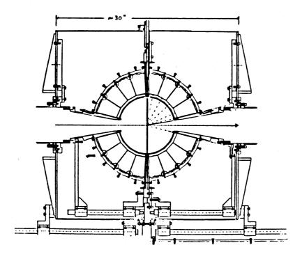
Figure 1. Schematic diagram of ISiS detector array.
