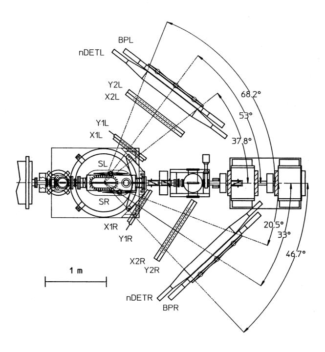
Figure 2. Schematic top view of the experimental setup. Protons are detected by a start scintillator (S#), two pair of x-y wire chambers (X#,Y#), a plastic scintillator array (nDET#) and additional backing plastics (BP#). Neutrons are detected only in the plastic scintillator array.
