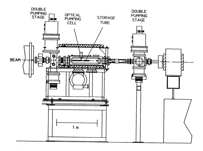
Figure 1. Side view of the polarized <sup>3</sup>He target. <sup>3</sup>He gas flows into a glass optical pumping cell, where it is polarized, and then to an open-ended storage tube in the vacuum chamber where the beam interacts with it. There are two pumping stages upstream and downstream of the target region in order to reach ambient Cooler vacuum. The beam enters from the left.
