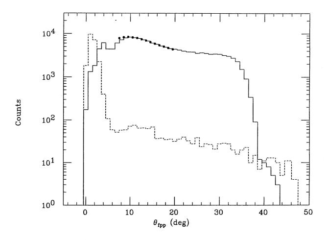
Figure 2. Angular distribution observed in the FPP. Solid (dashed) histogram is with (without) the small-angle rejection hardware activated. The dots represent the angular distribution from Ref. 2.
