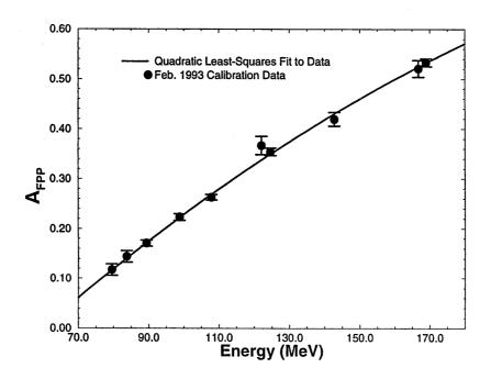
Figure 1.  $A_{FPP}$  versus energy for the first part of the E367 calibration data (see description in text).
