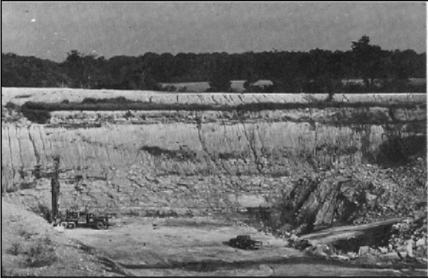
Figure 1. Thick overburden in a crushed stone quarry in Allen County, Ind.
