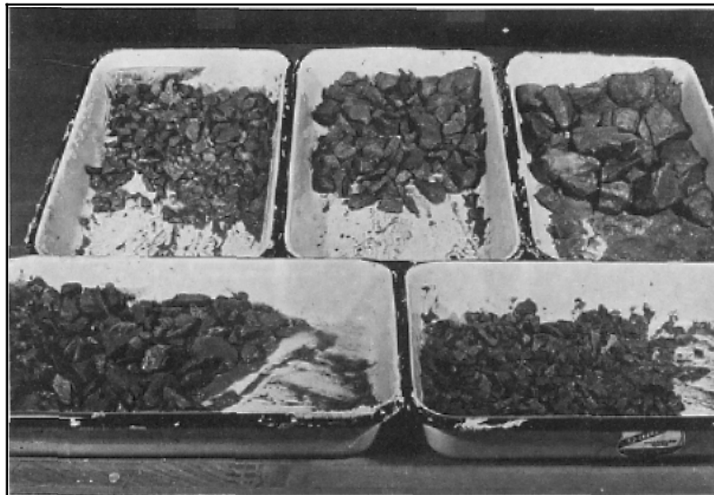
Figure 9. Five different sizes of a clay-rich dolomite (Saluda Formation) after the fifth cycle in a sodium sulfate bath. Percentage loss for all samples was 33.9~
