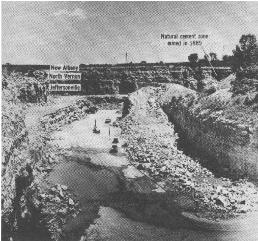
Figure 4. Adits of room and pillar mining operations in the North Vernon and Jeffersonville Limestones, Clark County.
