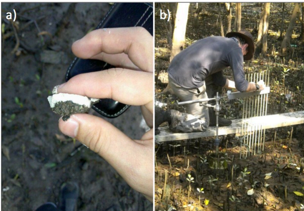
Figure 2: Slow rates of sediment accumulation eg over 1 year (a) can be measured precisely using the Rod Surface Elevation Table (b) - an instrument that is drilled into the bedrock and uses pins to measure millimetre change in mangrove sediment accumulation and/or loss at six-monthly intervals. This data can be easily converted into rates of carbon accumulation, and should be a method that is incorporated into all wetland PES schemes that monetise carbon sequestration.
