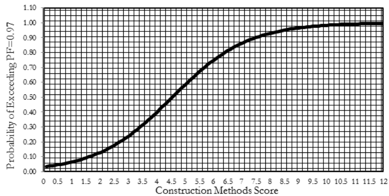
Figure 1: Probability plot of construction methods
