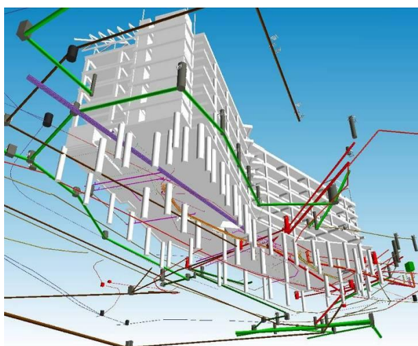
Figure 3 Utilization of BIM Model for Underground Utilities Coordination (Courtesy of: Holder Construction, Atlanta, Georgia, USA)
