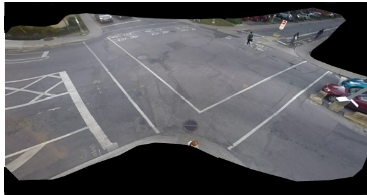
Figure 3-8 Mask to delineate the areas for detection and tracking (the area in black is not processed)
