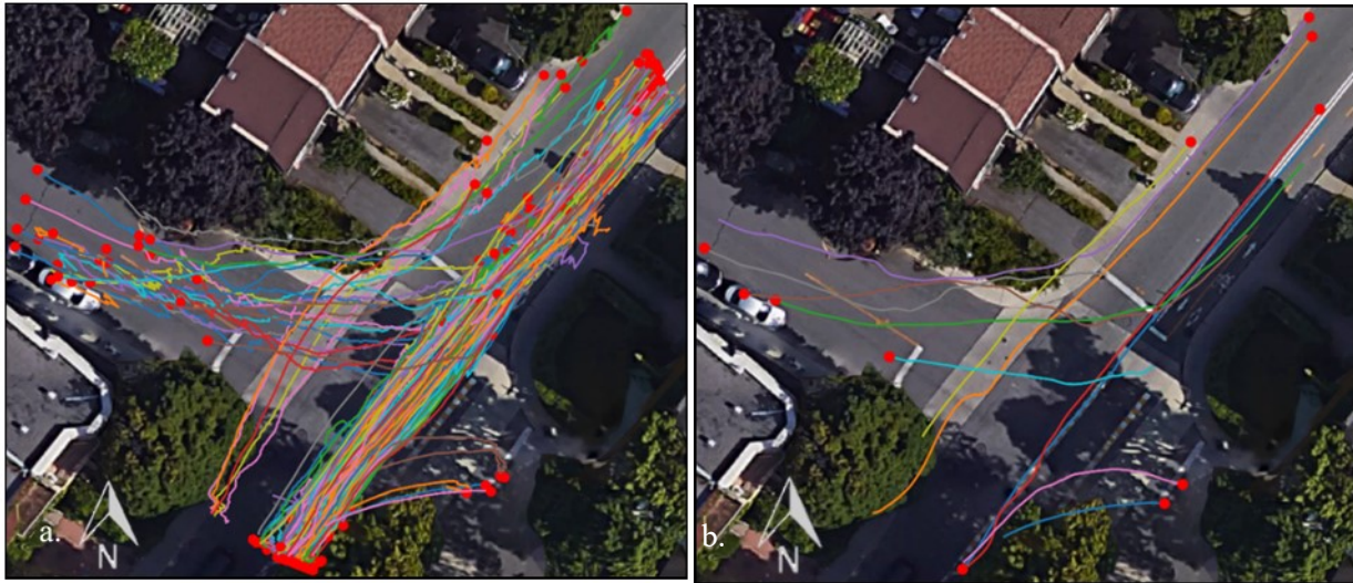
Figure 3-12 a. Cyclist trajectories, and b. cyclist motion patterns (origins marked in red circle)
