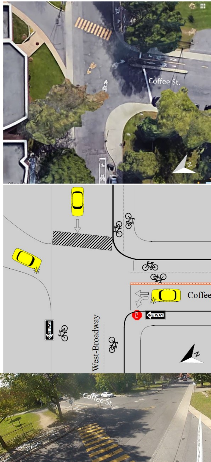
Figure 3-6 Continuous cycling facility on all legs: Coffee street and West Broadway street (Google Maps)
