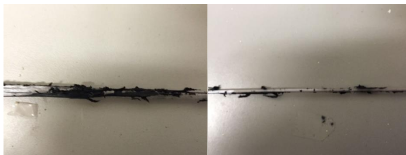
Figure 6.1: Photos of the drawn fiber (when the BTO concentration is higher than 30%).
