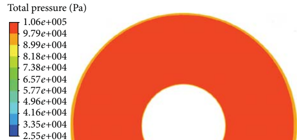
FIGURE 16: Contours of the total pressure obtained by a steady state calculation.
