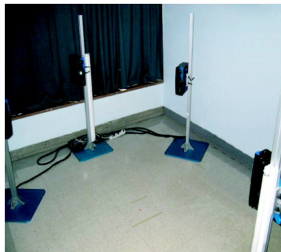
Figure 1 Inspeck system. Inspeck system used for capturing surface topography data. Four digitizers allow the capturing of the full surface of the patient torso.
