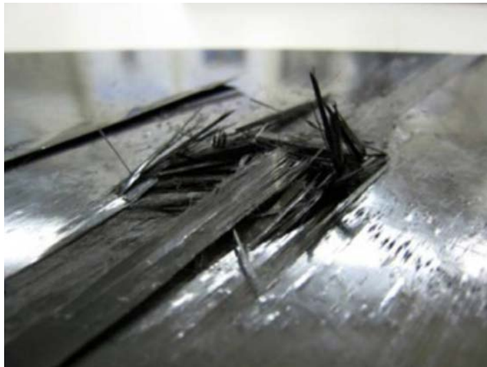
Figure 2.5: Typical lightning strike emulation damage to unprotected CFRP panel [10]. Fiber shortening is observed at the attachment point as well as lifted plies in the fiber direction. Resin blistering and swelling is also observed
