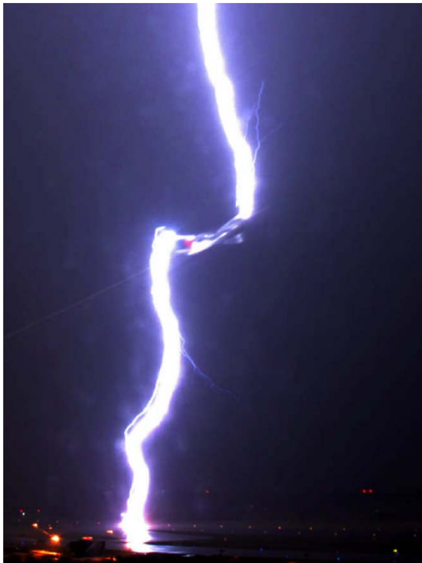
Figure 2.2: Aircraft-initiated lightning strike on takeoff. Leaders expanding away from plane can be clearly seen [16]
