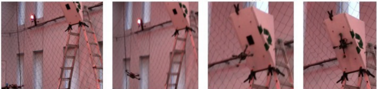
Figure 1.5 Problem Definition : Original results showing a quadrotor perching on a 120^\circ surface (taken from [1])
