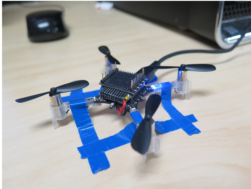
Figure 3.4 Test Bench for Accelerometer Variance Data
