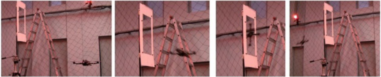
Figure 1.4 Problem Definition : Original results showing a quadrotor flying through a 90^\circ window (taken from [1])
