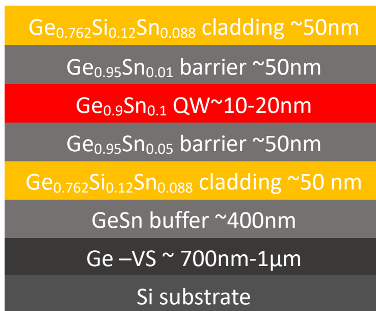
Figure 7-4: Direct band gap \text{Ge}_{0.9}\text{Sn}_{0.1} QW with type-I band alignment and carrier confinement
