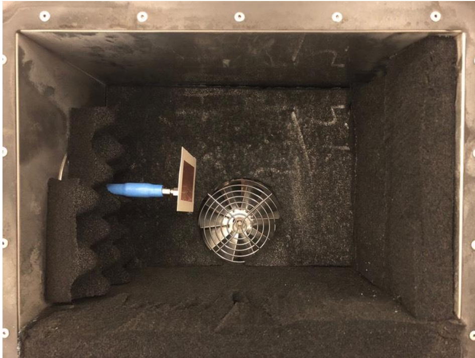
Figure 3.22 - Temperature chamber coated with the absorbers
