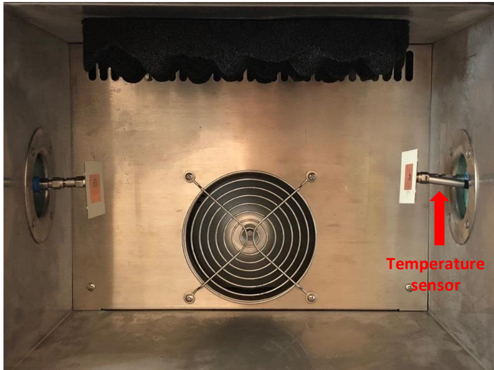
Figure 5.12 – Testing signal transmission of wireless temperature sensor network system
