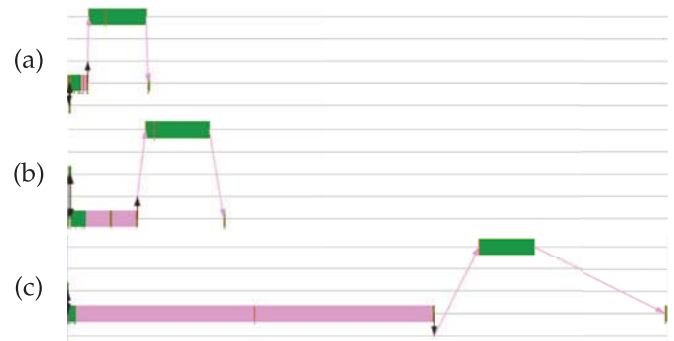
Fig. 4. Active path of wk-rpc according to the network latency. The execution in (a) has natural network latency, in (b) the latency is set to 10 ms and in (c), the latency is set to 100 ms.
