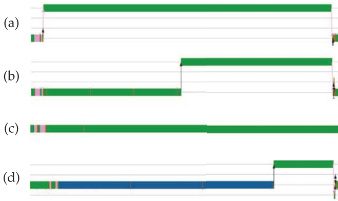
Fig. 5. Active path of wk-rpc according to asynchronous processing level of 0 percent in (a), 50 percent in (b) and 100 percent in (c), and asynchronous processing based on event loop in (d).
