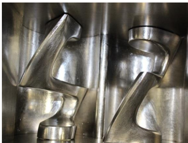
Figure 2.15: Interior of the sigma type mixer shown in Figure 2.16
