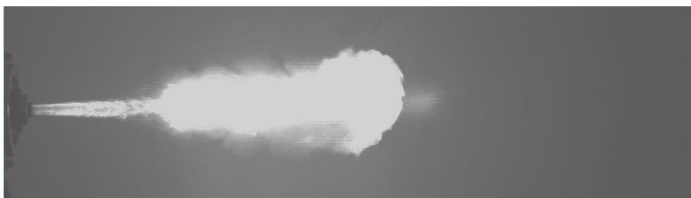
Figure 7.3: 35% BTA propellant vented vessel flash
