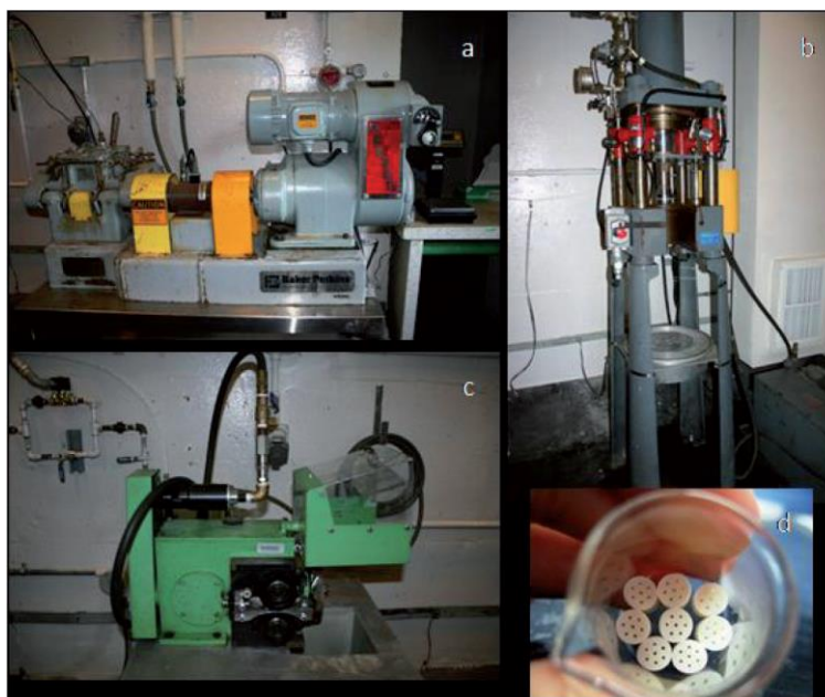
Figure 2.16: Propellant manufacturing facility [76] a) sigma mixer, b) extrusion press, c) cutting machine, d) 7 perforation propellant grains.
