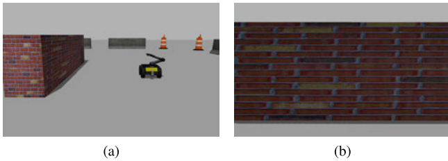
Fig. 2. (a) Starting configuration for the robot and camera with respect to the structure. (b) Initial image seen by the camera: the robot only knows that the structure in the FOV is the one that should be mapped.
