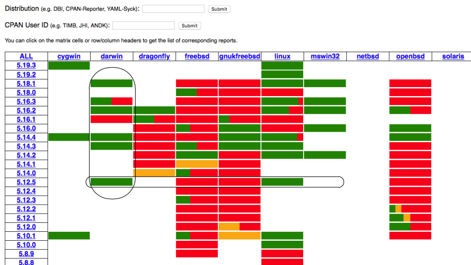
Figure 4.1 Example of CPAN build report summary. A vertical ellipse represents an “environment build vector” (RQ3), while a horizontal ellipse represents an “OS build vector” (RQ4).
