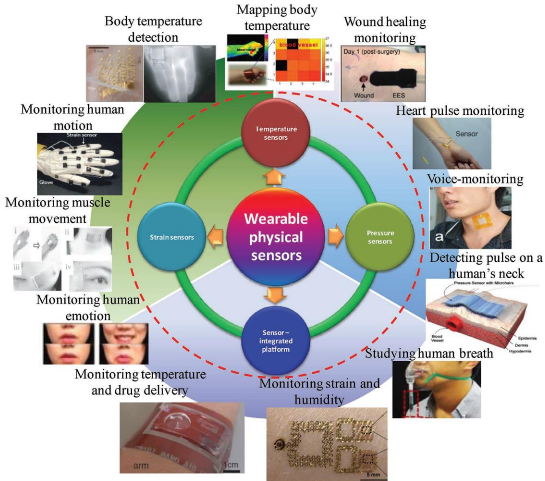
Figure 2.15: Characteristic properties of recently developed wearable physical sensors for monitoring human activity and personal healthcare [98]
