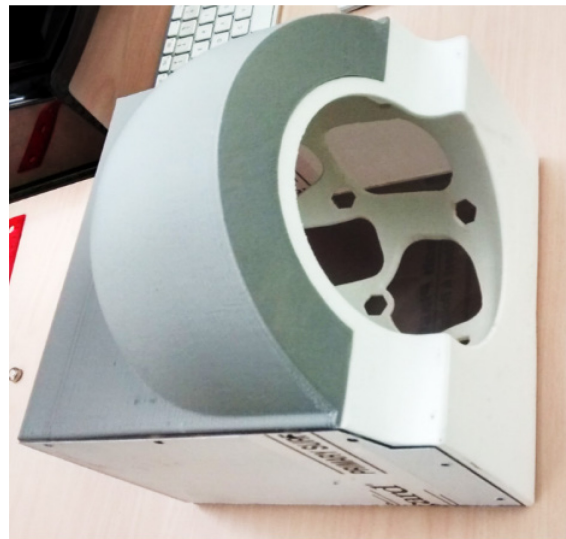
Figure 4.21 Picture of the coil housing with the spherical frame, which is also a part of the external assembly.
