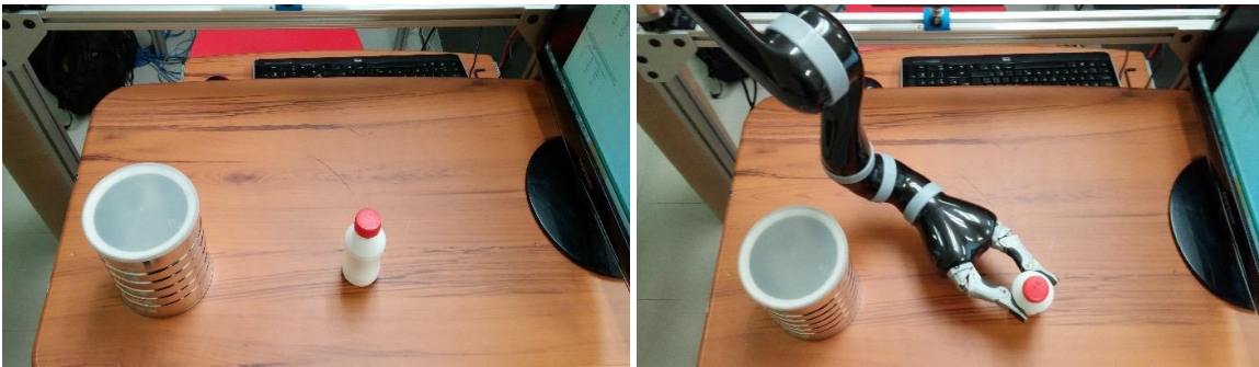
Figure 5-8 Position of the object of interest and the obstacle (left). Object of interest grasped by the JACO arm (right)
