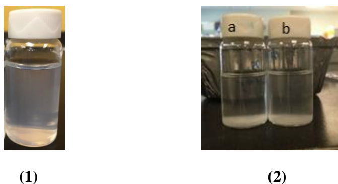
Figure 4.4. The dispersion state of 1) pristine CNC 7 and 2) modified CNC with Chitosan in DI water (a) CHI1000-CNC (b) CHI87-CNC.
