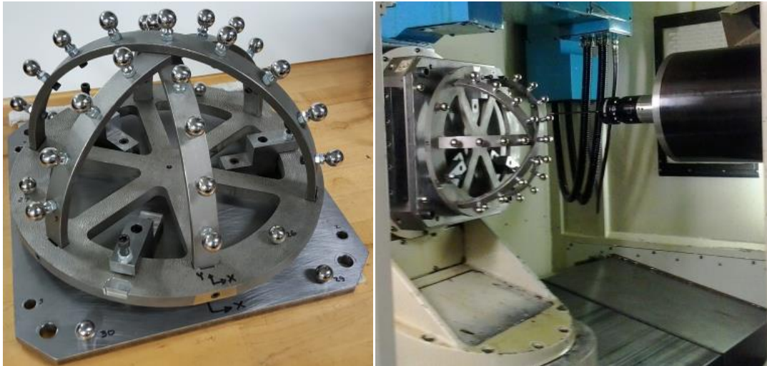
Figure 4.1: Photos of the ball dome artefact (left) and loaded on the C-axis of the machine tool ready for probing (right)
