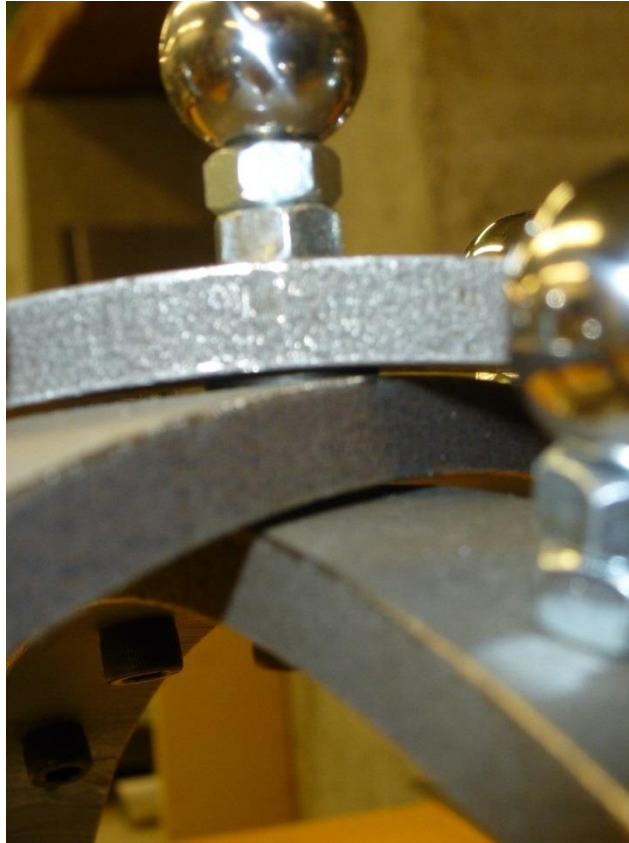
Figure 5.6: Attaching the arcs together in the mid-point
