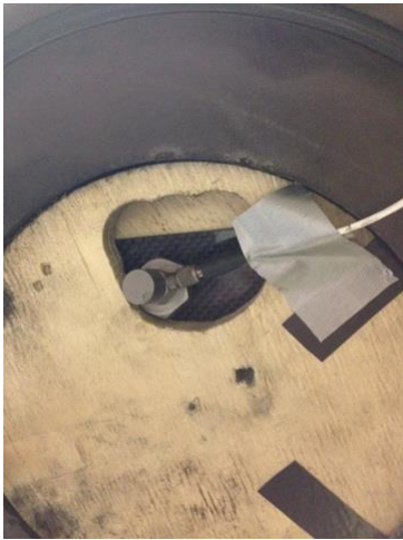
Figure 4.10: Accelerometer mounted on sample
