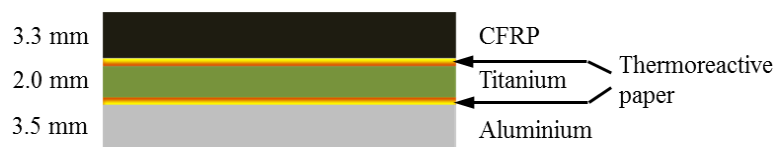
Figure A-2: Stack material specifications
