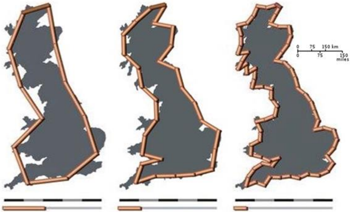
Figure 2-15: Fractal analysis evaluating the British coastline length using different stick lengths (Andrus, 2005)
