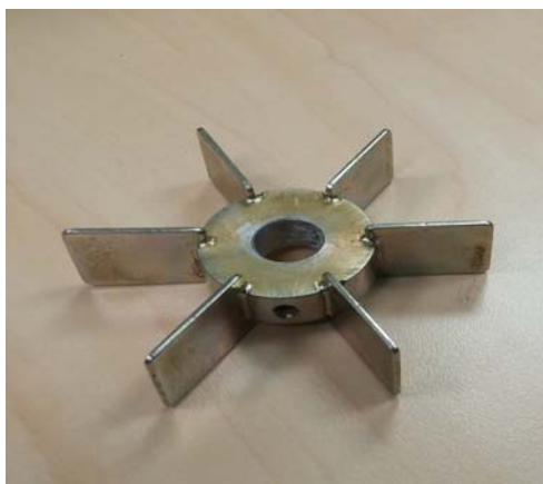
Figure 4-2: Rushton turbine impeller with six vertical blades used in this study (outside diameter: 5.0 and 7.5 cm for reactors R1 and R2, respectively)
