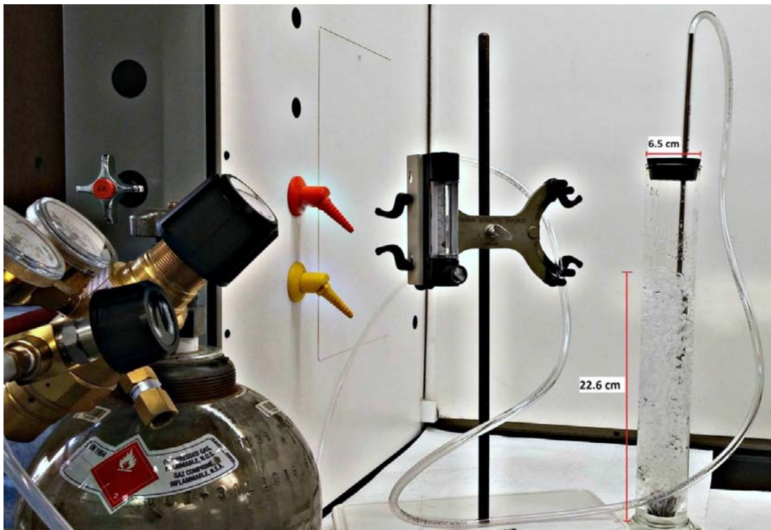
Figure 4-6: Photograph of the set-up used in the H 2 stripping batch test
