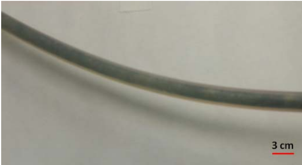
Figure 5-4: Black precipitate observed on the inside wall of the tube (1/4 in ID \times 3/8 in OD) transferring mixed liquor from AN reactor to the OX reactor (Phase # 3B)
