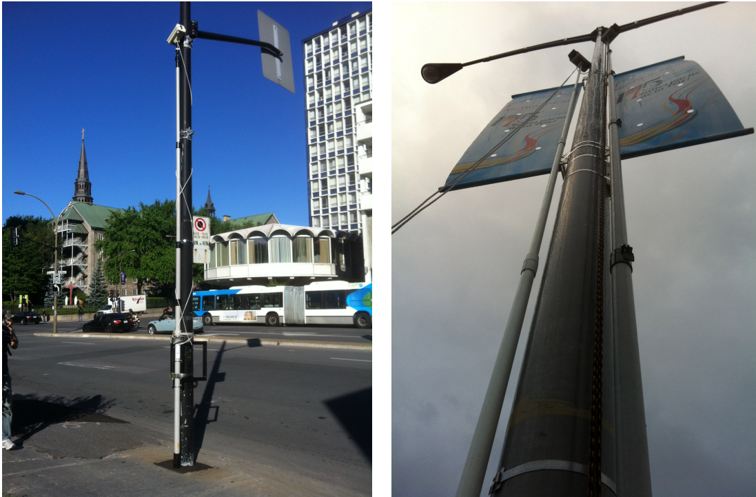
(a) VCU deployed at reduced height near an intersection (b) Two VCUs deployed at full height near a roundabout, for full coverage.
