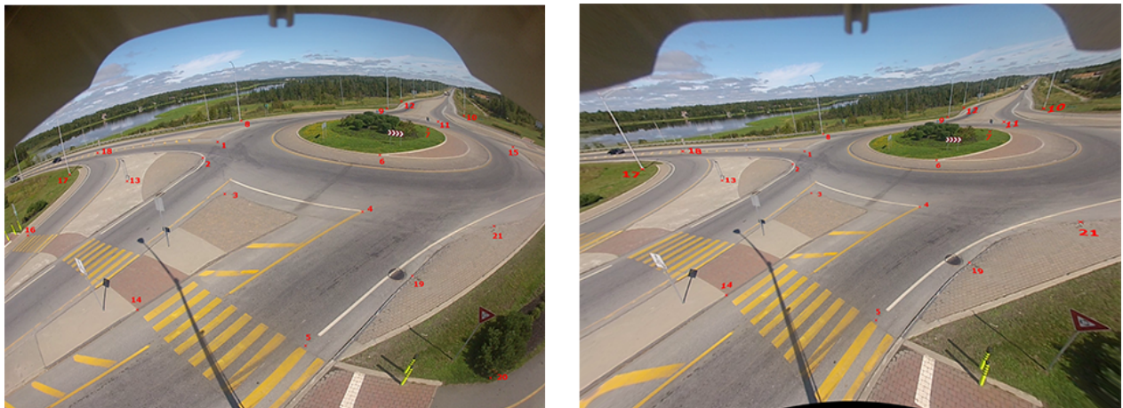
Figure 3.3 Side-by-side comparison of image before (left) and after (right) lens distortion correction.
