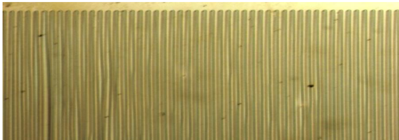
Figure 3.9: Inverted domain pattern in lithium niobate after etching under the microscope.
