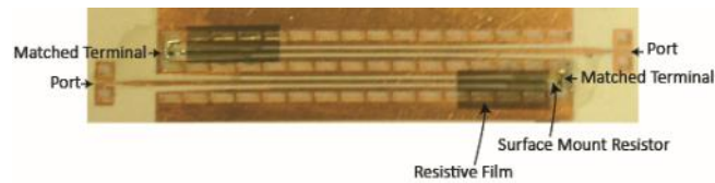
Figure 5.10: Fabricated circuit for crosstalk measurement.
