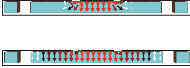
Figure 4.2: Intended modes in MSTL with the dominance of vertical electric field components: a) microstrip line mode, b) waveguide TE 10 mode.
