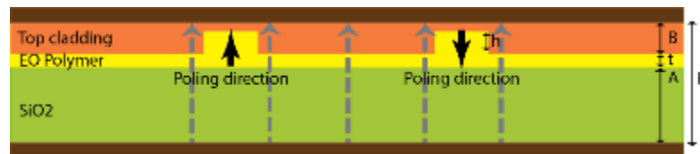
Figure 2.3: Cross-sectional view of the second proposed device showing the push-pull operation in a polymer EO MZM. Black and gray arrows represent poling and modulation field directions, respectively.
