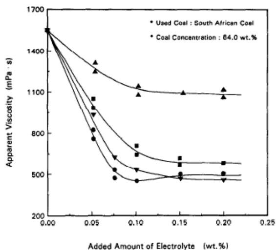
**Figure 3** Influence of type and amount of electrolyte on the viscosity of CWM. Additive: CWM 1002, 0.4 wt.%. Electrolyte: ▲,  $Mg(OH)_2$ ; ■,  $Ca(OH)_2$ ; ▼,  $KOH$ ; ●,  $NaOH$
