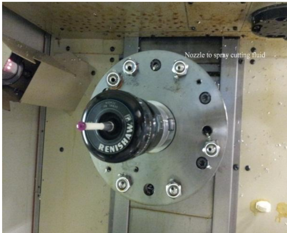
Figure 7-3 Spindle with nozzle to spray cutting fluid holding the probe
