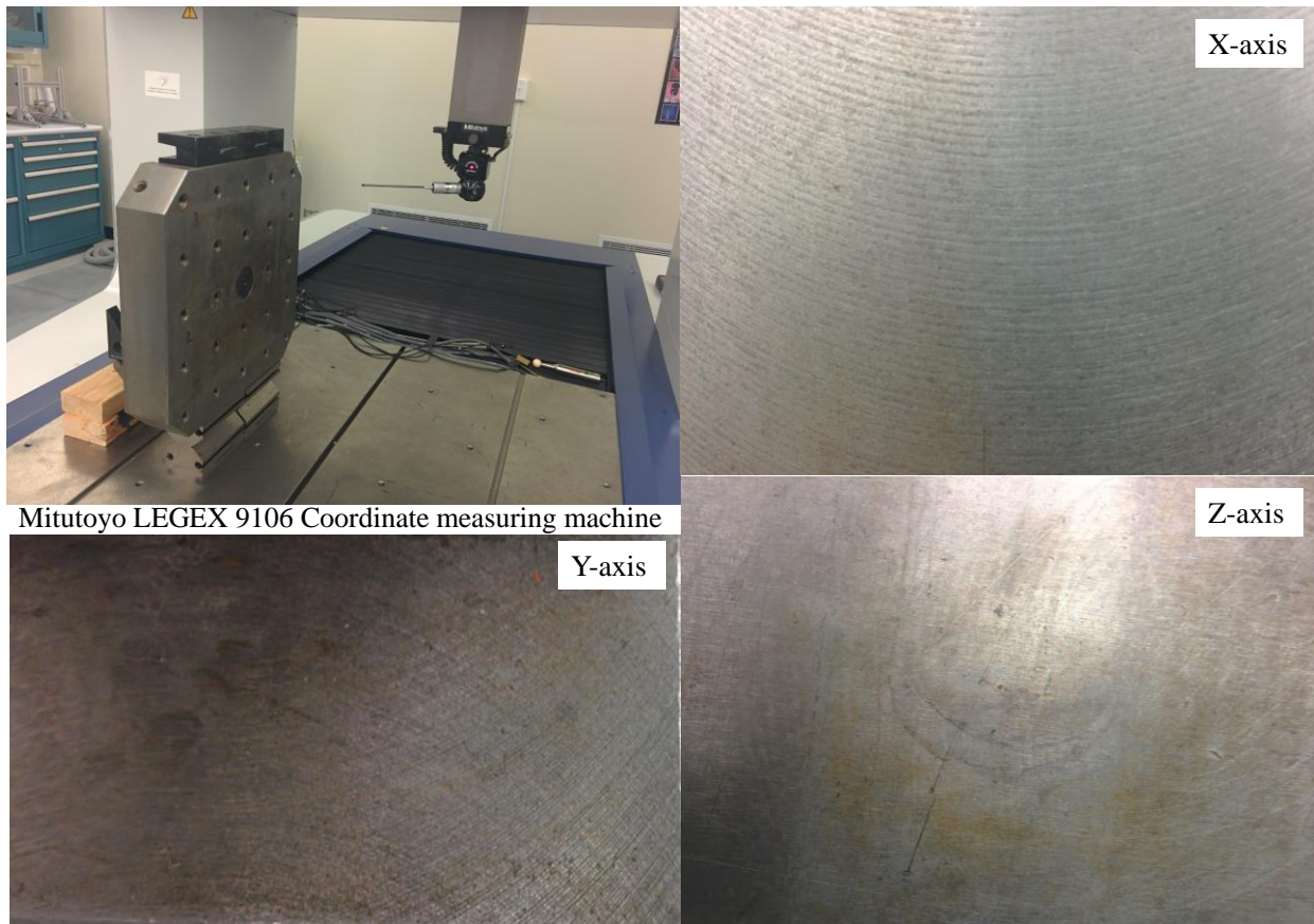
Figure 7-8 The Coordinate Measuring Machine (CMM) and surface quality at X-, Y- and Z-direction
