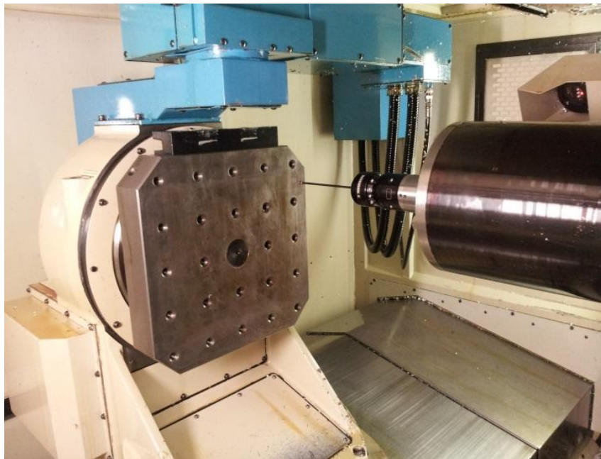
Figure 4-1 Machine table, of a WCBXFZYST five-axis machine tool, used as indigenous artefact for probing
