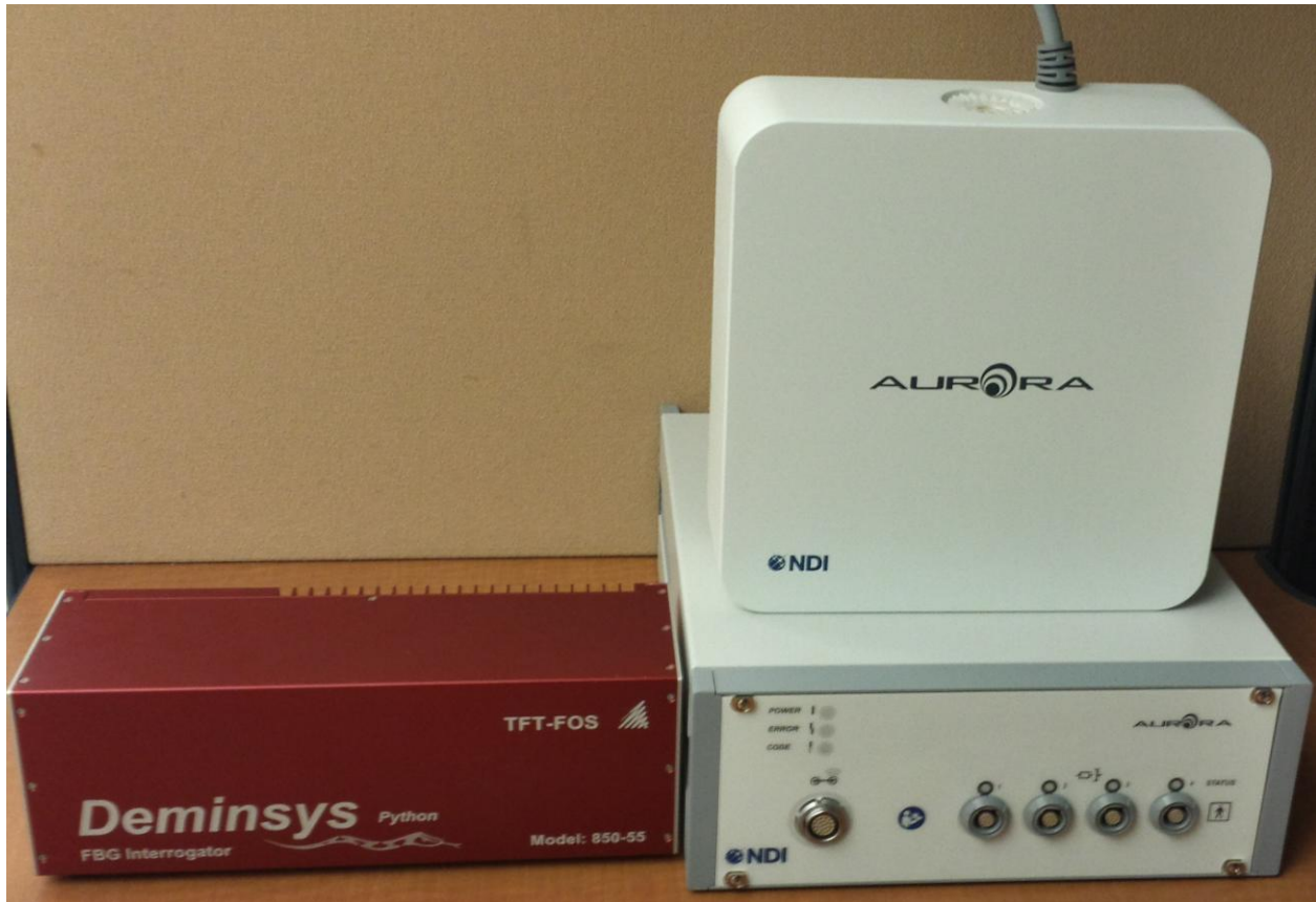
Figure 6.3: Side-by-side physical dimension comparison between a Deminsys® interrogator and an Aurora field generator with its system control unit.
