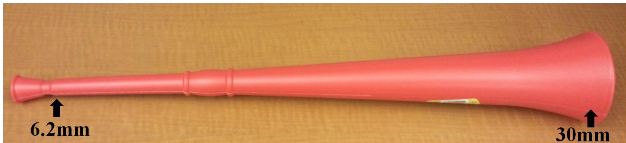
Figure 6.6: A cylindrical cone shaped plastic object with an inner diameter ranging from 6.2 mm to 30 mm.
