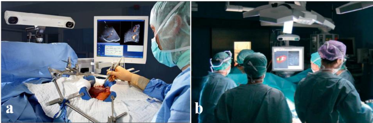
Figure 3.4: Application of OTS in the operating room: (a) Polaris localizer camera used to track a surgical instrument in an image-guided liver resection procedure [46], (b) NDI Vicra, a passive OTS mounted in an operating room [47]. Used with permission.
