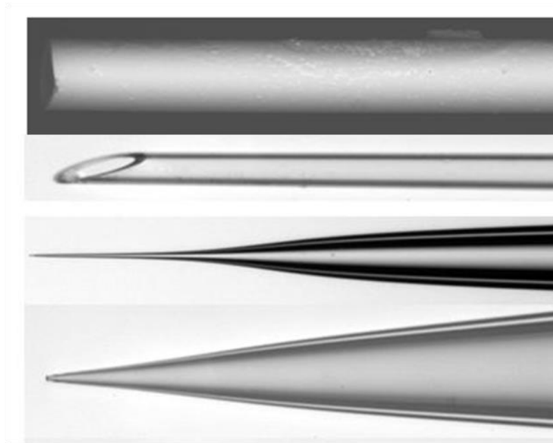
Figure 2.3. SEM (top) and Optical microscopy images of pre-processed and conventionally processed glass pipettes. Reprinted with permission from Ref. [15].
