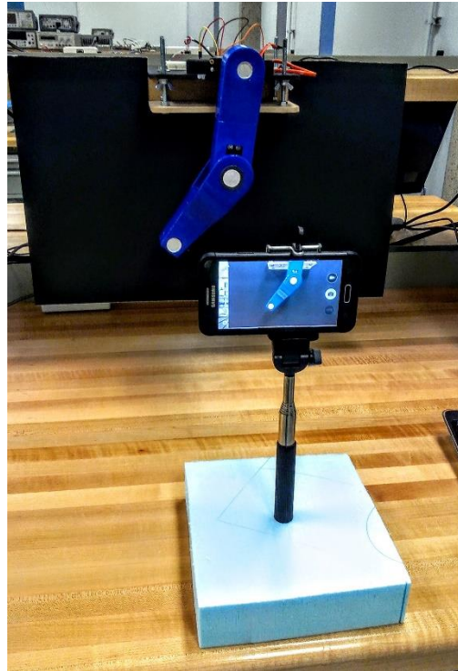
Figure 7.7 : Kinematic acquisition using a smartphone video camera, reducing both costs and difficulty while keeping the experimental part of the project
