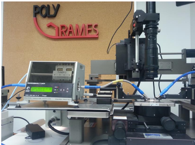
Figure 4-10: Picture of part of the setup used to compare the PCE of the HSMS-2850 and backward tunnel diode. The picture shows the probe station and the Focus Microwaves Tuner, used as matching network.
