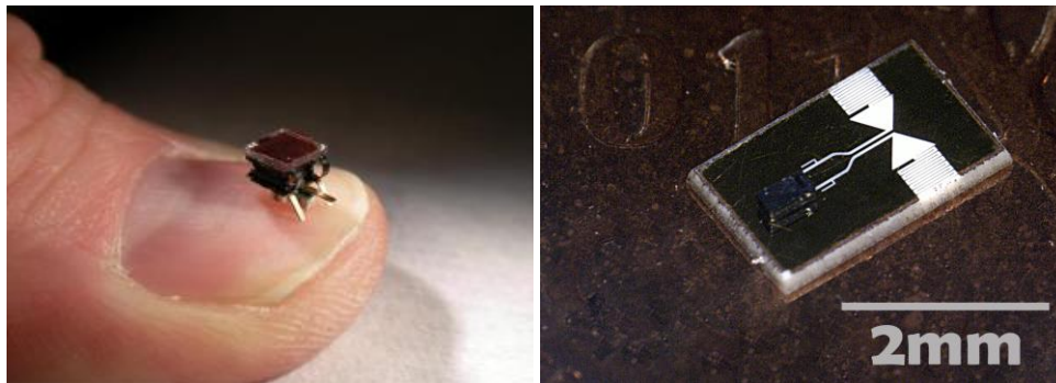
Figure 5-1: (a) Photograph of the I-SWARM micro-robot [77], (b) Proposed 94GHz rectenna.
