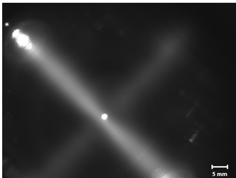
Figure 5.22: Cloud of ^{85}\text{Rb} in a MOT taken from top-view with the CCD astro-camera. The cooling beams and magnetic field were aligned to produce the ideal, uniform distribution in space.
