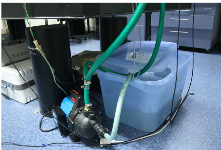
Figure IV.1: Photo of the 35 m of head waterpump and its connections to the water reservoir and up toward the coils.
