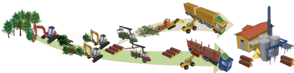
Figure 3-8: Hybrid harvesting system with hogfuel grinding at cutblock roadside ( modified image, original courtesy of Forest Energy Portal [136] )
