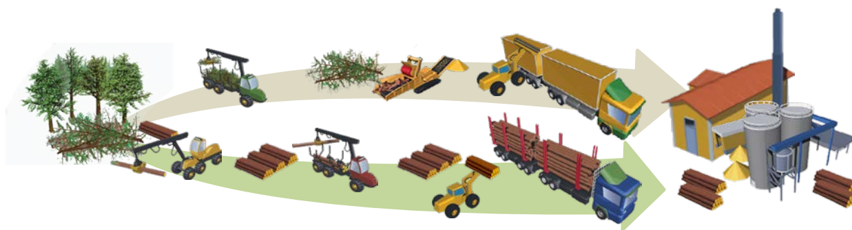
Figure 3-6: Cut-to-Length harvesting system with hogfuel grinder at cutblock roadside ( modified image, original courtesy of Forest Energy Portal [136] )
