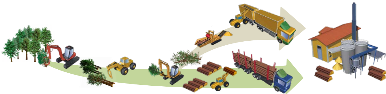
Figure 3-7: Full-tree harvesting system with hogfuel grinder at cutblock roadside ( modified image, original courtesy of Forest Energy Portal [136] )
