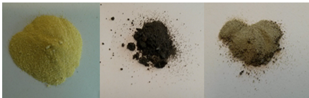
Figure 4.11 Al-V-Mo (a) before reaction, (b) after reaction (continuous system) (c) after reaction (oxidation-reduction system), T = 650 \text{ K} , C_{\text{O}_2} = 0.04 .
