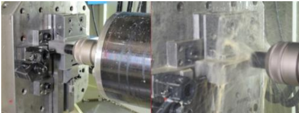
Figure 5-2: Lubricated face milling with carbide inserts
