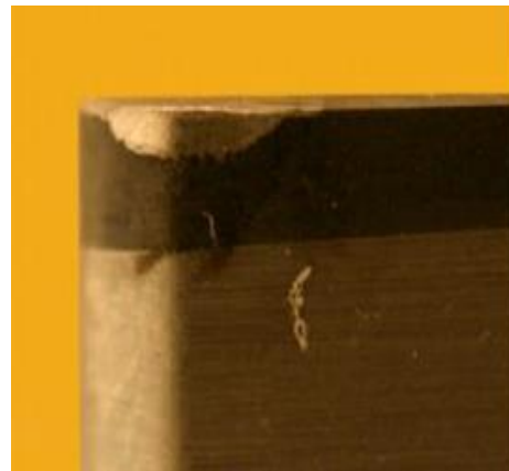
Figure 4-13: Flank wear of CBN insert under following cutting conditions Cutting volume 15,973\text{mm}^3 v_c=150\text{m/min} ; f_r=0.3\text{mm/rev} ; a_p=0.1\text{mm}
