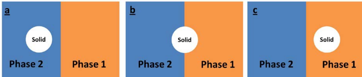
Figure 2.13. Different localizations of solid inclusions based on the wetting parameter( \omega ): (a) in Phase 2 when \omega > 1 ; (b) at the interface when -1 < \omega < 1 ; (c) in phase 1 when \omega < -1 .
