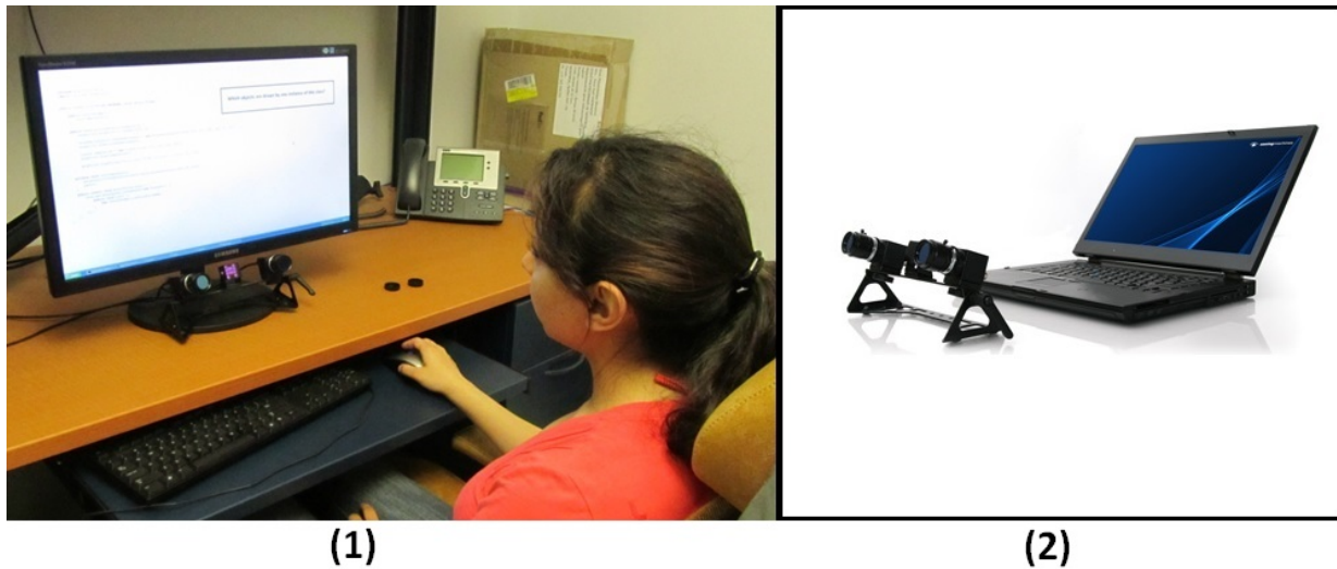
Figure 2.2 1) FaceLAB is an example of video-based eye-tracker that we used in this work (adapted from FaceLAB manual (Seeing Machine, 2010)). 2) Participant sits in front of the computer and a video-based eye-tracker captures the eye-gaze data.
