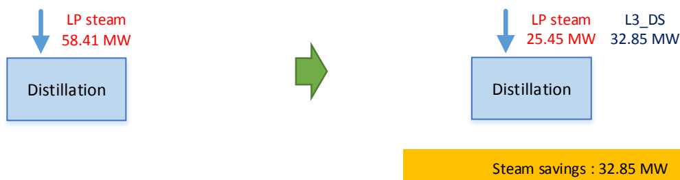
Figure 5-11 Comparisons of the LP steam consumptions between the project A (stand-alone) and the IFBR A
