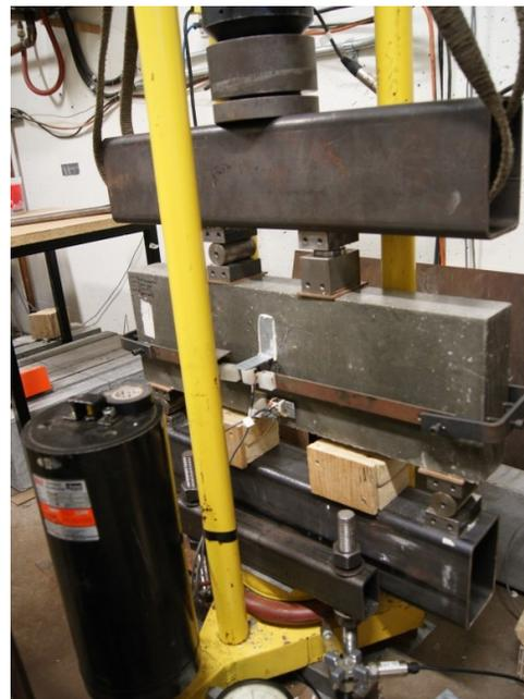
Figure 4.2 : Sustained loading test apparatus
