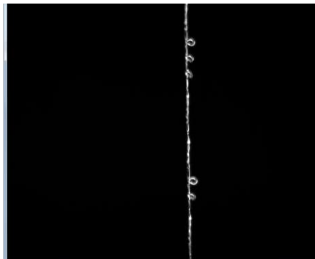
Figure 25: Supplementary Video 4: Video of tensile testing of ISCP-made fibers (Batch F). Bonds break one after each other. The video is interrupted before the rupture of the backbone.
