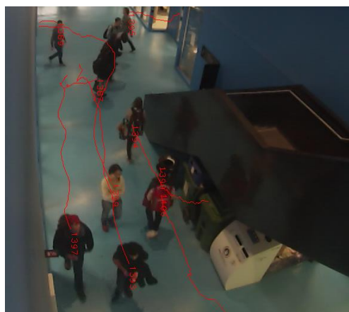
Figure 4.11 Example frame of Traffic Intelligence tracking on the Polytechnique calibration sequence.
