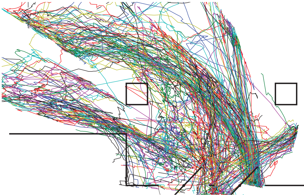
Figure 5.2 Trajectories produced by optimized Traffic Intelligence for a 30 minute sequence in the subway station scene.
