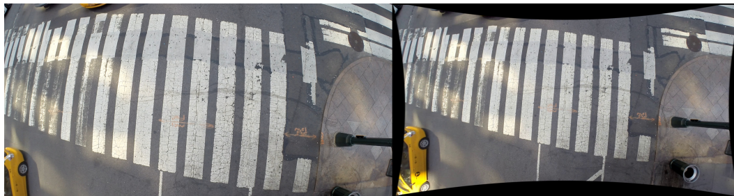
Figure 3.2 Lens distortion in the New York video sequence (left) and the same frame after correction by the tool included with Traffic Intelligence (right). Note that though these frames are presented at the same size for clarity, the left one is 1920x1080 pixels, whereas that after correction is 2515x1415 pixels.
