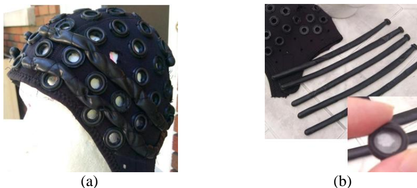
Figure 5-2. A regular cap lined with tube balloons : (a) The positioning of the tube balloons on the cap, (b) The shape of tube balloons used and the filtration ring that secures the granular material inside the balloon during air pumping
