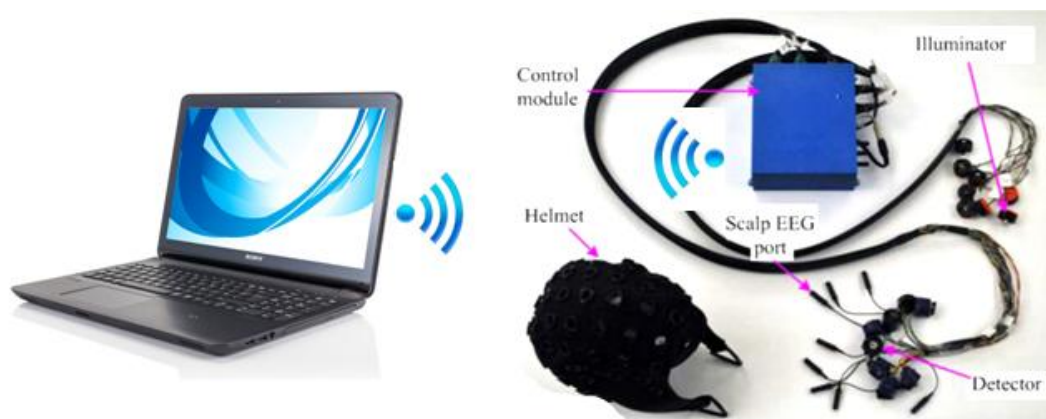
Figure 1-2: Combined EEG/NIRS portable system developed by the Imaginc group of Polytechnique Montreal. The brain device interface represents the combination of optodes and the helmet used to stabilize them, these are wired to the control module that can be fixed on the belt. Data collected in the control module are transmitted via Bluetooth transmission to a laptop where signal processing takes place in real time
