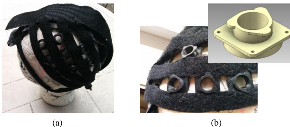
Figure 5-3. Velcro bands lined with tube balloons: (a) General distribution of the balloons and optodes, (b) The special socket design in order to increase the stability of the optode
