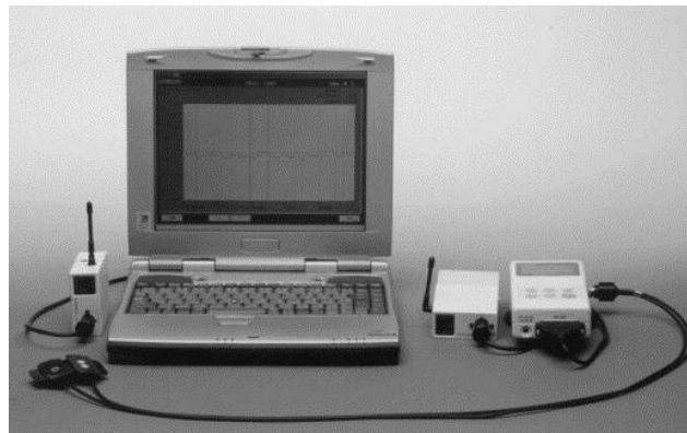
Figure 2-1: Example of a Wireless NIRS device (Hoshi & Chen, 2002)
